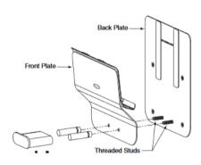
4. Remove Front-Plate from Back-Plate by pulling the Front-Plate off the threaded
